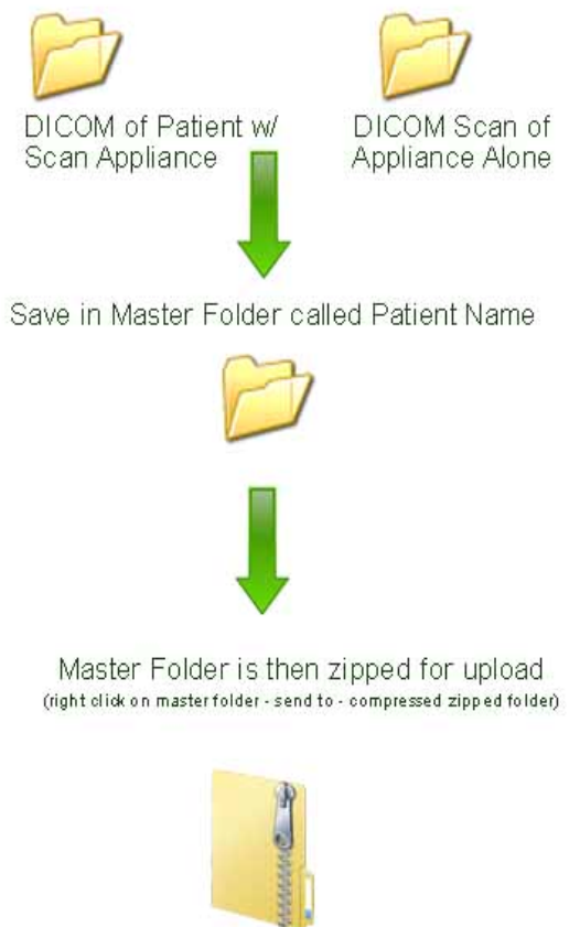
Figure 4 – A sample of the file structure that should be saved and uploaded to ROE.
